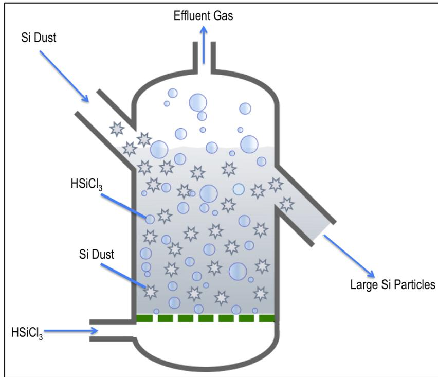
**Figure 2.** Fluidized Bed Reactor
